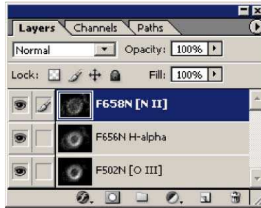
Fig. 26.— The layers palette in Photoshop with all three image layers. Note that the layers have been renamed for clarity. Six layers will be present if the highlights and shadows layers for each dataset are not flattened into single layers for each dataset.
