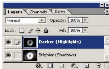
Fig. 21.— The layers palette in Photoshop for a single file that contains the two images from Figure 20. The darker image that shows the details in the bright regions of the nebula is in the layer on top. The brighter image that shows the detail in the faint regions is in the bottom layer. Note that the top layer is currently selected, which means that all editing will affect only the top layer. Also note that visible layers are marked with an eye on the left of the layer.
