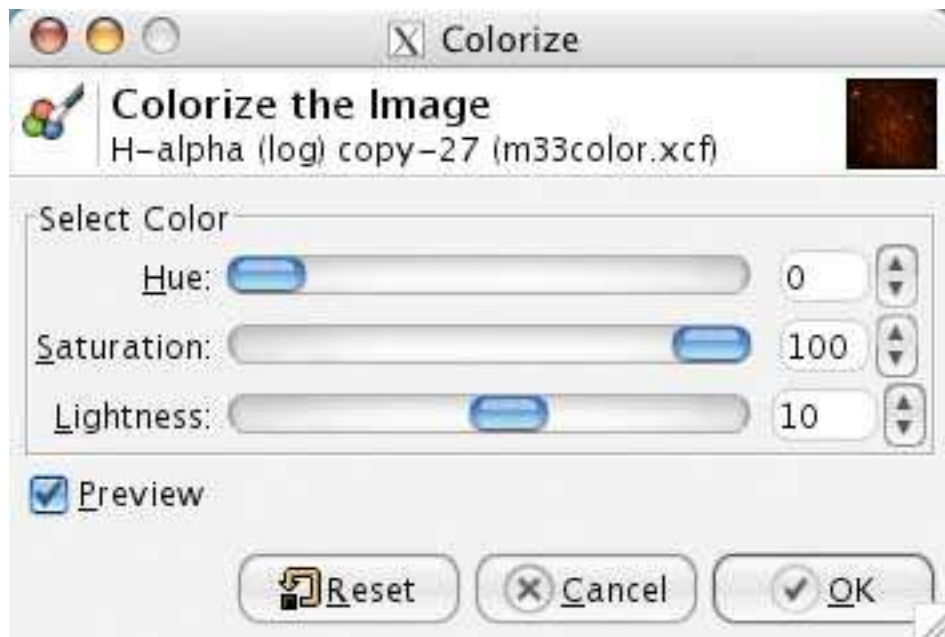
Fig. 18.— An example of the Colorize dialog box in The GIMP. Here it is set to give the H\alpha layer a red color ( 0^\circ in hue).
